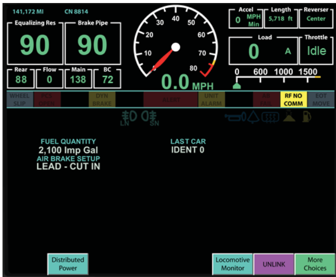
EMD Gauges Screen (Main Operating)
