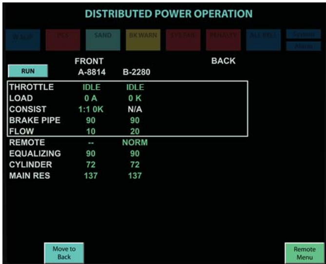
EMD Distributed Power Operation Screen
